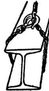
3. No direct binding of a load with a load chain
