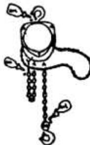
8. Do'nt forget to oil the load chain after use
