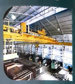
50/20 TON X 12 MTR. SPAN CRANE FOR SLR STEEL BANGLORE
