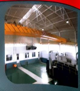
20 TON X 17 MTR. SPAN CRANE FOR UNITECH MACHINES
