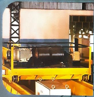
Rope Drum: It is made of steel on which wire rope grooves are accurately machined for proper sitting of wire Rope. Specially designed arrangement is provided so that Wire Rope changing is very easy without involving any clamping or tightening on the drum.
