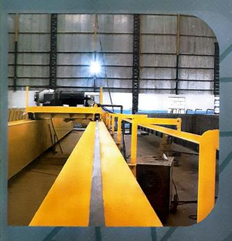
10 TON X 17 MTR. SPAN CRANE FOR FRONTIER ALLOYS
