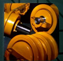
Steel forged deep hardened on the rail surface insures the ultimate resistance to wear with maximum roller life. Double self align spherical bearing housed with L- blocked wheel assemblies
