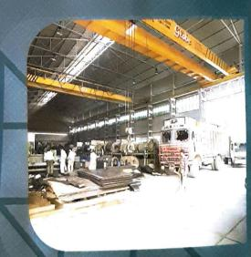
15 TON X 18 MTR. SPAN CRANE FOR UNITECH MACHINES
